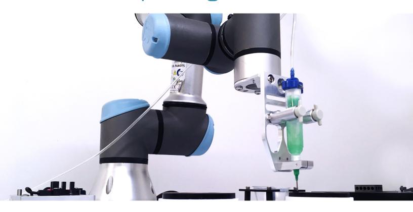
Robot27's Dispense is part of our growing lineup of precision material dispensing end effectors for robots. Three models enable the pneumatic dispensing of adhesives, lubricants, solvents and more. Each model comes with everything you need to quickly and easily set up your robot for dispensing. Simply load a material cartridge onto the end effector, connect the air supply, and start your robot program.
