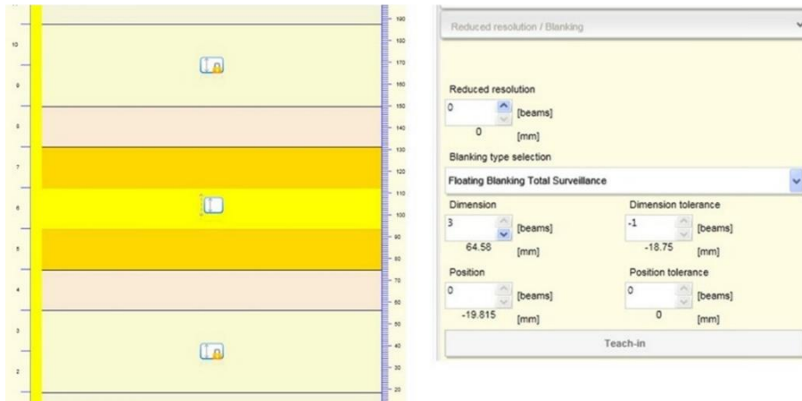
Fig 96 - Floating blanking with total surveillance
