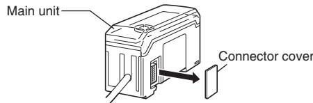
**2 Install the amplifiers (expansion units) on the DIN rail.**
