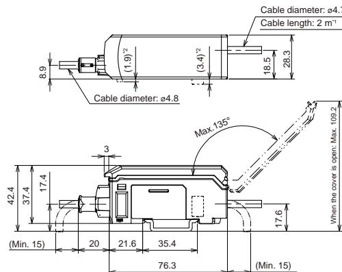
\*1 Cable specification : IL-1000 12 cores, Nominal cross-section area brown/blue: 0.20 mm<sup>2</sup>, others 0.15 mm<sup>2</sup>
