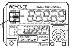
The tolerance setting value can be set either manually or automatically.
