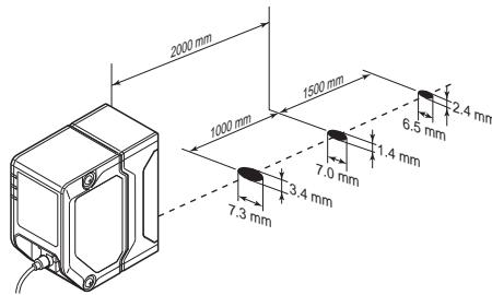
The optical axis may vary by approximately  $\pm 1.5^\circ$  (IL-2000), or  $\pm 2.0^\circ$  (IL-030/IL-065/IL-100/IL-300/IL-600).
