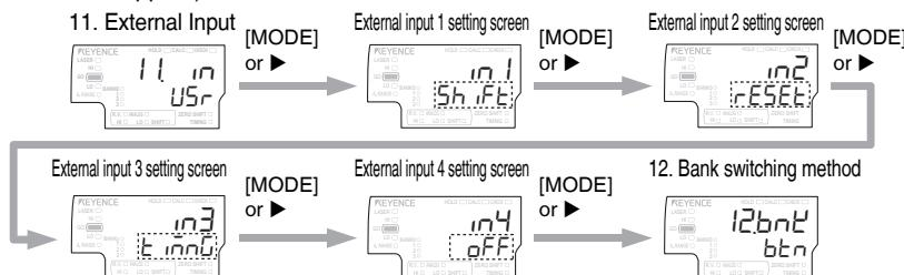
Press **▲** / **▼** button on each setting screen to specify functions.
