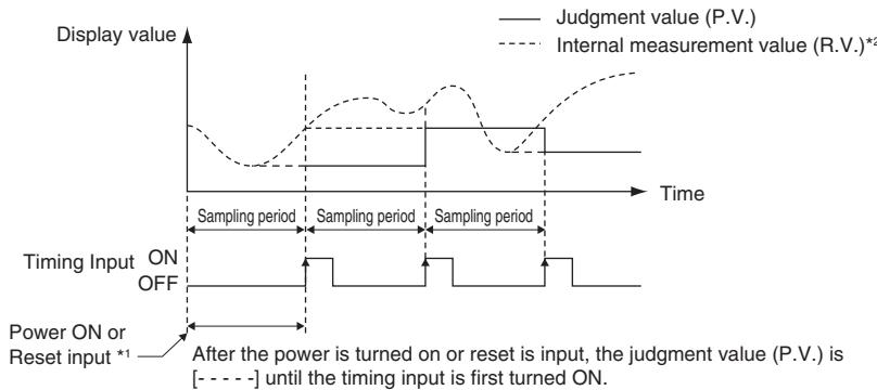
Power ON or Reset input \*1 After the power is turned on or reset is input, the judgment value (P.V.) is
