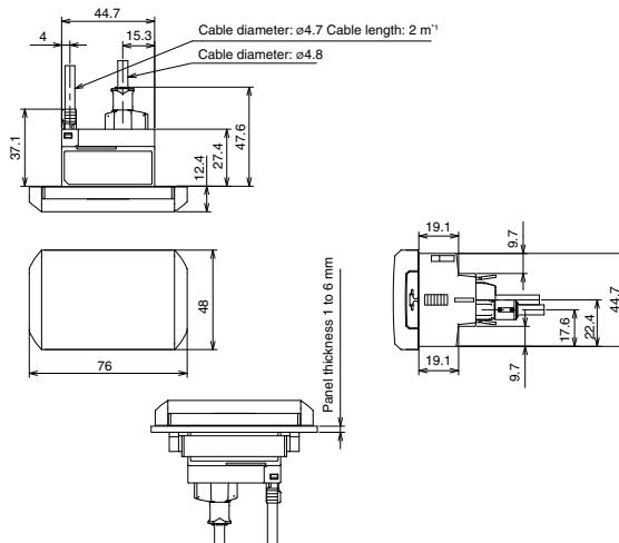
\*1 Cable specification : IL-1000 12 cores, Nominal cross-section area brown/blue: 0.20 mm<sup>2</sup>, others 0.15 mm<sup>2</sup>
