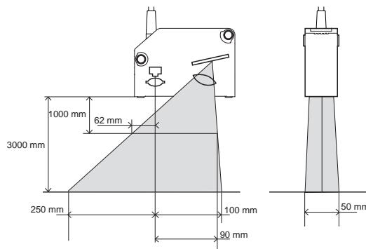
This drawing shows the interference area when the optical axis is perpendicular to the target surface.
