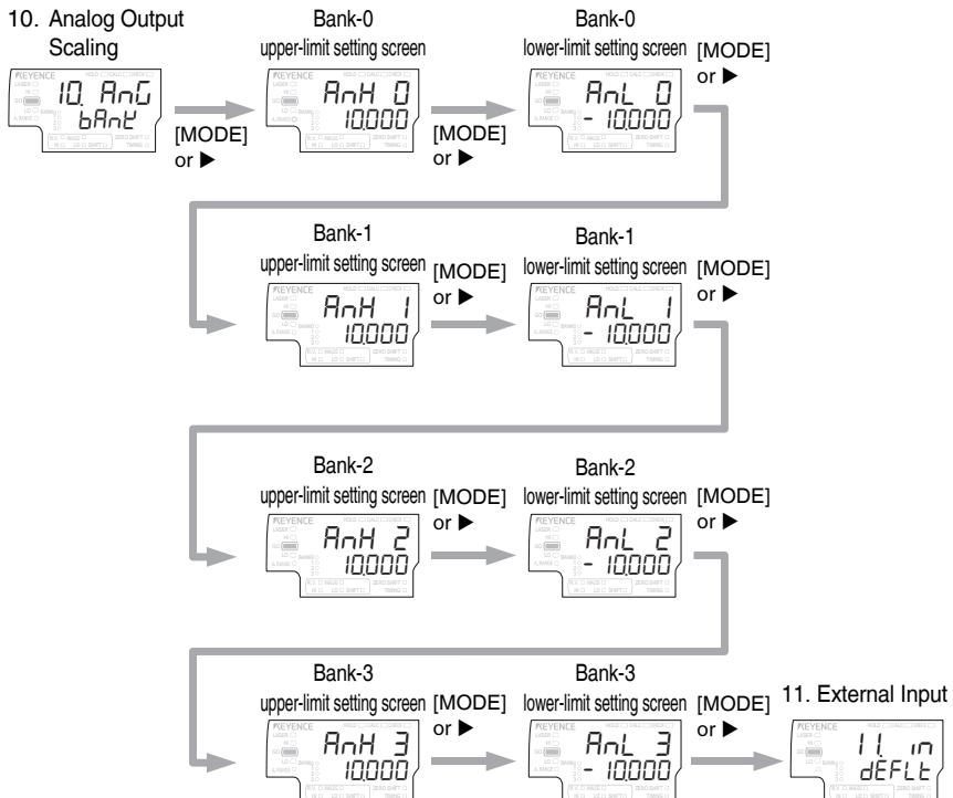
Press  $\blacktriangle$  /  $\blacktriangledown$  button on each setting screen to specify the upper limit and the lower limit.
