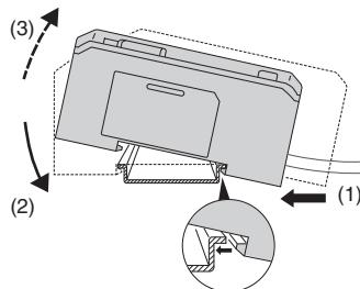
**2** To dismount the sensor, raise the main body in the direction of the arrow (3) while pushing the main body in the direction of the arrow (1).
