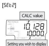
**6** Insert workpiece B for which the measured value is known, and using the  $\blacktriangle$  /  $\blacktriangledown$  buttons, set the "CALC you wish to display (2)" for that workpiece B.
