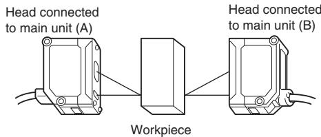
If the zero shift function is used, the actual diameter or width of the object can be displayed as a calculation value (CALC value).
