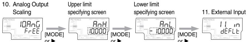
Press  $\blacktriangle$  /  $\blacktriangledown$  button on each setting screen to specify the upper limit and the lower limit.
