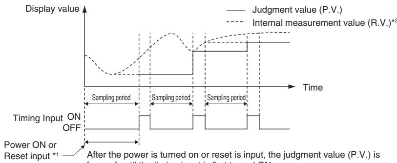
Power ON or Reset input \*1 After the power is turned on or reset is input, the judgment value (P.V.) is
